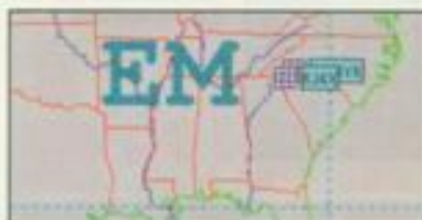
Figure 1—This is a simulation of the 2-meter band "at rest" (147.585 MHz), as viewed from BEACONet station KJ4X. Notice that only icons representing local stations appear on the map.
