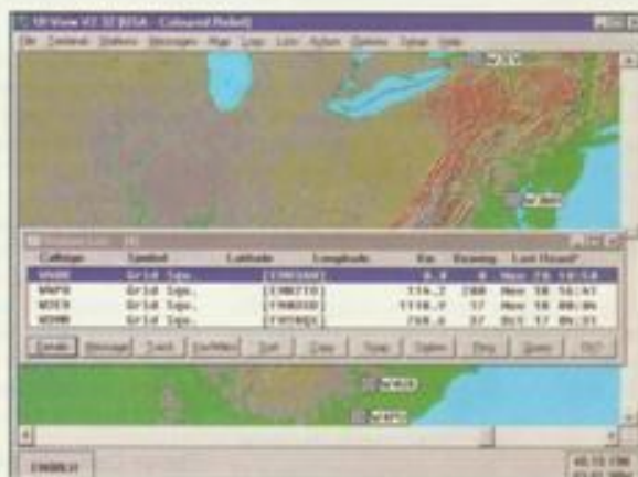
Figure 3—An actual BEACONet screen shot from W4UK showing successful receptions of 147.585 MHz transmissions made during the November 2000 Leonid meteor shower.
